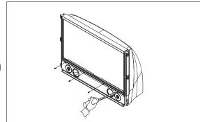
4. Loosen the screws. Remove the front mask.
