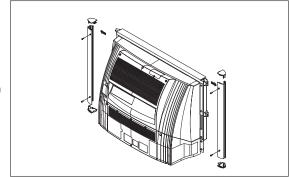
2. Loosen the screws and remove the supporter.
