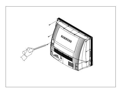
2. Loosen the screws and remove the supporter.
